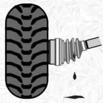
Unfortunately, trail imperfections, ice build-up, hard turning, stretching, or aging can cause the CV boot to rupture. This allows road debris
